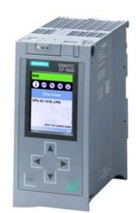
SIMATIC S7-1500, CPU 1515-2 PN, CENTRAL PROCESSING UNIT WITH WORKING MEMORY 500 KB FOR PROGRAM AND 3 MB FOR DATA, 1. INTERFACE: PROFINET IRT WITH 2 PORT SWITCH, 2. INTERFACE: ETHERNET, 30 NS BIT-PERFORMANCE, SIMATIC MEMORY CARD NECESSARY
